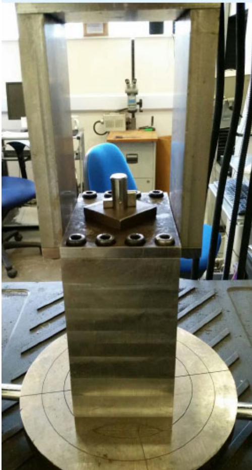
Figure 3.1 Static tension test arrangement
